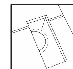
For heating vents, cut the plank to length, measure and mark areas to cut out, then cut allowing for expansion.
