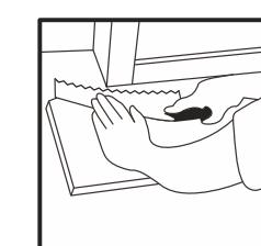
Trim door frames by placing a plank upside down next to the frame and cutting to the necessary height.
