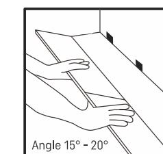
Assemble the second row on the subfloor, tilt and push to attach to the first row, then click into place.
